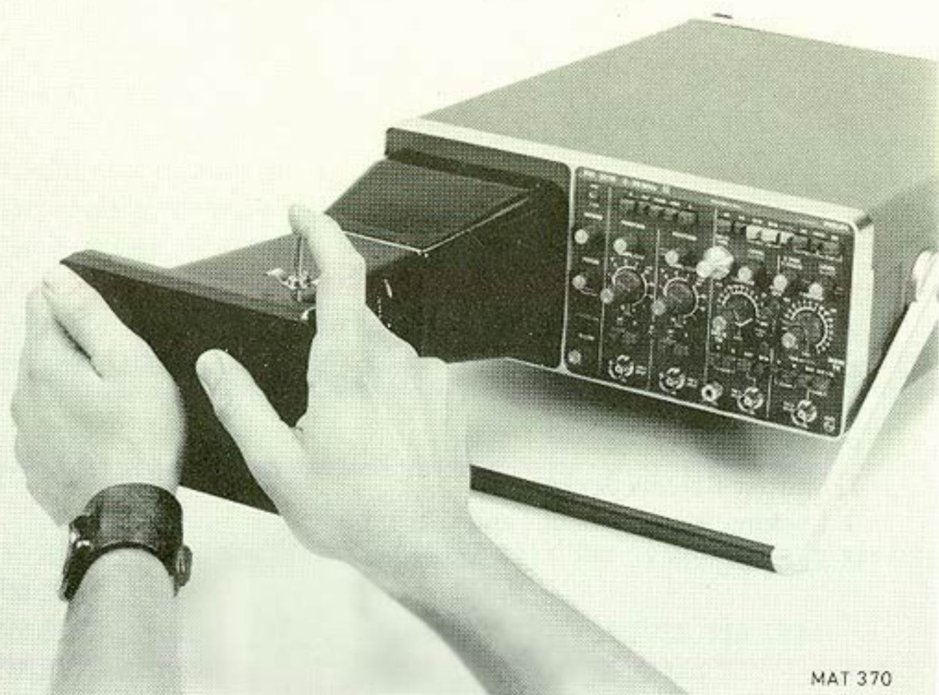
Fig. 4. Holding camera and hood in position over oscilloscope bezel during
